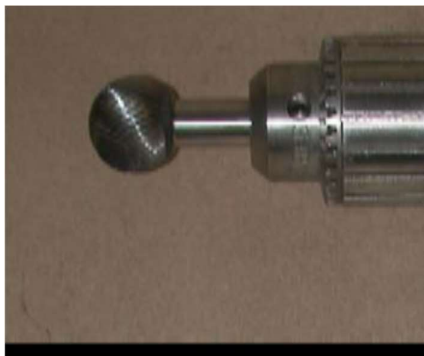
Figure 4: Photograph of typical spherical carbide ball burr
